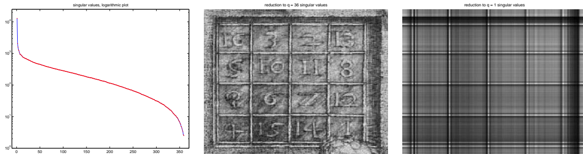
Figure 2: Logarithmic plot of the 359 singular values of the matrix of gray values of the pixels of the detail (left) and reconstructions of the detail using 36 (middle) and only 1 singular value (right). Apparently, the grid is the most dominant feature in the picture.
